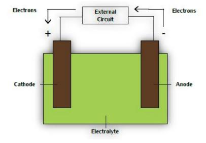
Fig. 01 – Circuit diagram of a galvanic corrosion cell<sup>2</sup>
