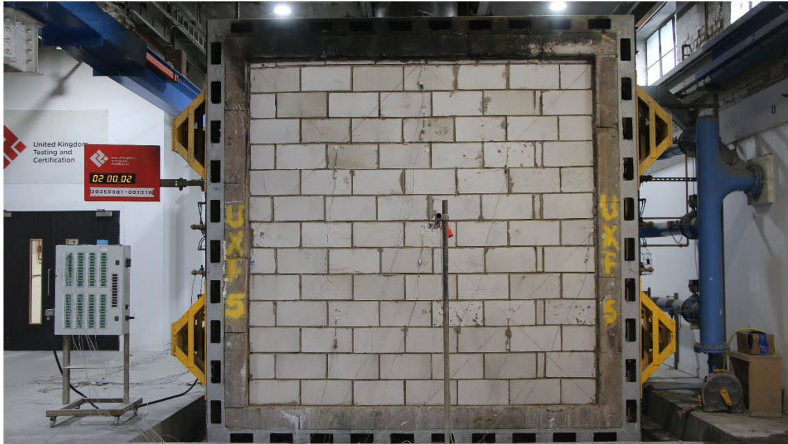
Figure 24 – The unexposed surface of the test construction after a test duration of 120 minutes
