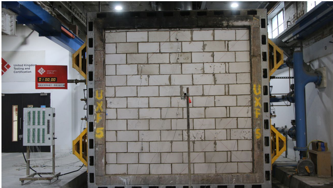
Figure 20 - The unexposed surface of the test construction after a test duration of 60 minutes
