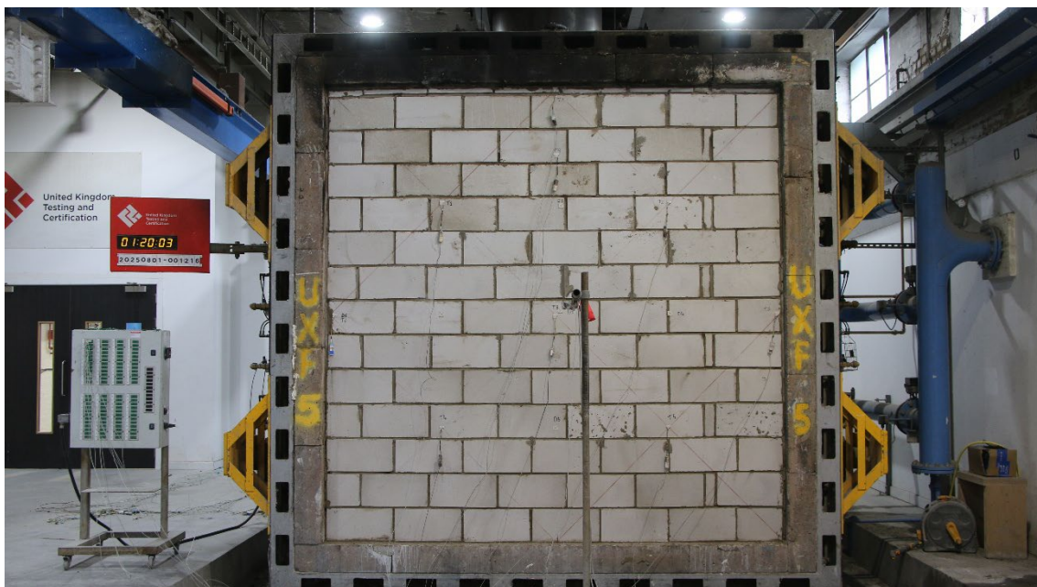
Figure 21 - The unexposed surface of the test construction after a test duration of 80 minutes
