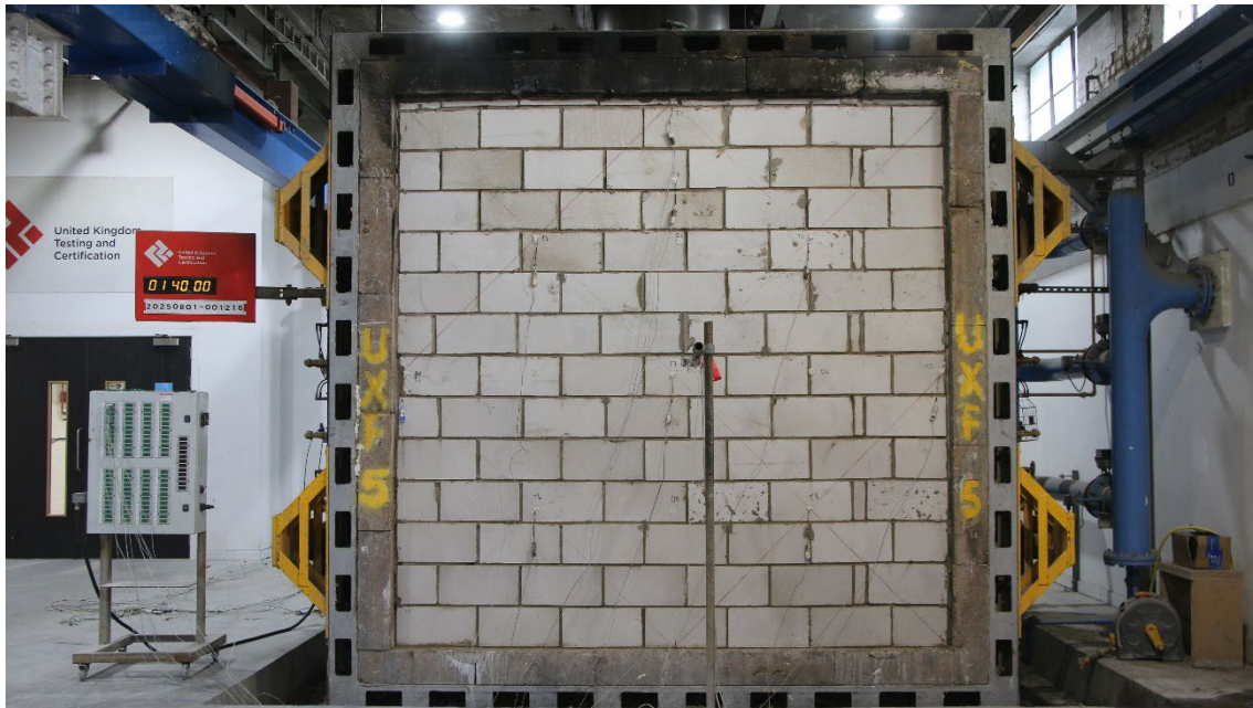
Figure 22 – The unexposed surface of the test construction after a test duration of 100 minutes
