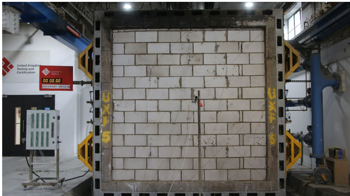
Figure 17 – The unexposed surface of the test construction prior to the commencement of the test
