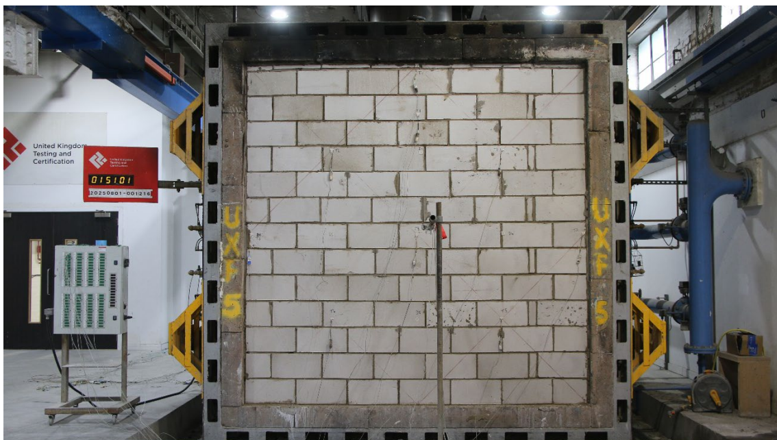
Figure 23 – The unexposed surface of the test construction after a test duration of 110 minutes
